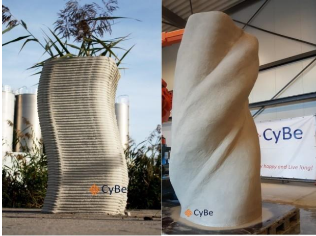
Fig. 6 Examples of freeform structures printed in concrete using a robotic arm successfully executed in 2015 and under further development
