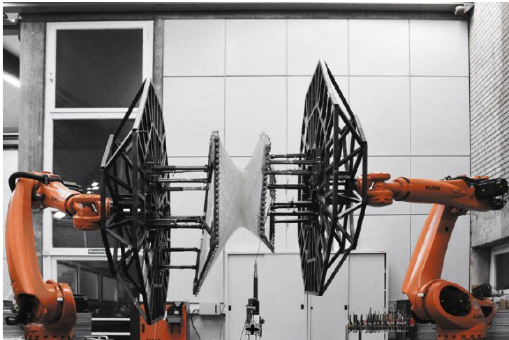
Fig. 1. Tridimensional form finding with carbon fiber structures using industrial robotic arms at the University of Stuttgart
