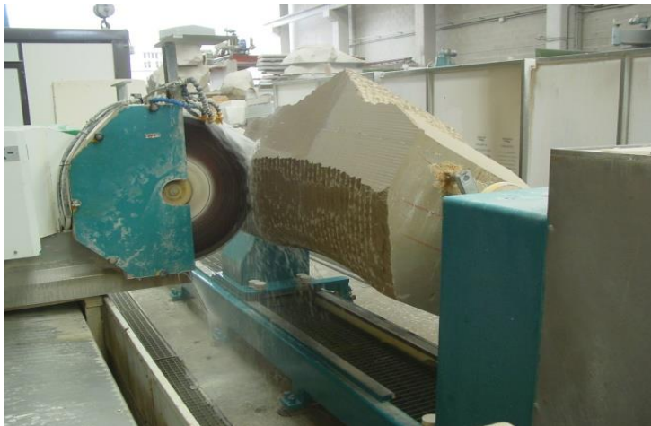
Fig.2 Horizontal pivot numerically controlled and machine specially adapted for the fabrication of a stone component of multiple ruled surfaces for the Basilica of the Sagrada Família
